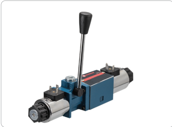
FWS can work as standard solenoid directional valve, also can control the spool movement with hand level on power-off condition.
