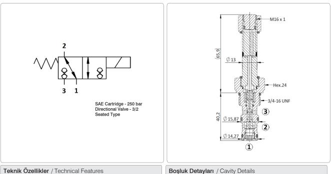
All external surfaces are zinc plated and corrosion-proof. All valve parts are made of high strength steel. Poppet is hardened and micron finished to ensure minimal wear and extended service life. Coil seals protect the solenoid system. Manual override option. Industry SAE common cavity.
