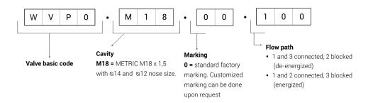
Note: All Solenoid cartridge valves listed in the present catalogue are designed to work with D.C. power supply. To work with A.C. power supply, a RAC coil and connector with rectifier must be used. For any additional information, please contact your Sales contact representative.
