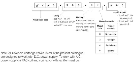
are designed to work with D.C. power supply. To work with A.C. power supply, a RAC coil and connector with rectifier must be used. For any additional information, please contact your Sales contact representative.
