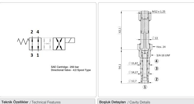
All external surfaces are zinc plated and corrosion-proof. All valve parts are made of high strength steel. Spool and cage are hardened and super-finished to ensure minimal wear and extended service life. Coil seals protect the solenoid system. Industry SAE common cavity.
