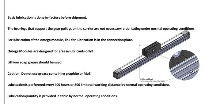
After lubrication, move the linear module along the stroke distance at least three times. Meanwhile, the moving speed should not exceed 10 mm/s.
